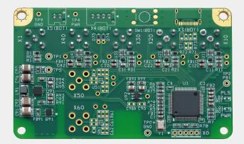
X1 (input) – input trigger (SMA through hole, straight). On board 0732513140 (Molex). Mating connector for cable 73251-0450 (Molex).
